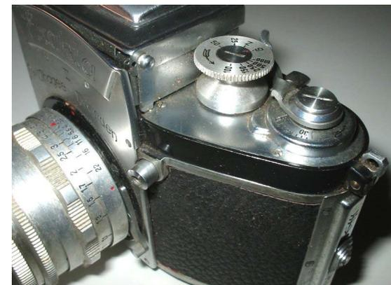
In the version 2 you can see how the upper part of the front plate was shaped to ensure more rigidity. The lens flange is black aluminium. On this camera you can see a big grain leather instead of the usual fine grain leather. The shutter fires while the curtains move slowly or stay open. Cosmetically good.
