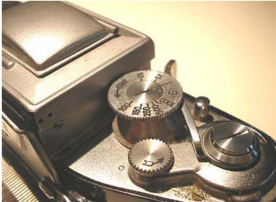
You can easily identify this camera because of the setting 1/150 second. The film pressure plate is removeable with stippled embossing.
