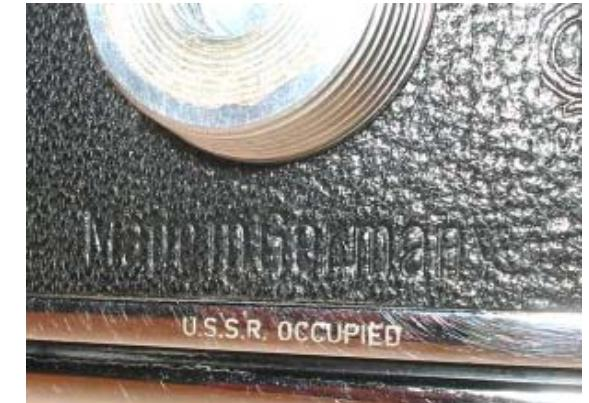
Exakta II A, #900772, version 4. This camera is the rare version 4 of the Exakta VX IIa. The front plate was hammered under the embossed inscription "Varex IIa", then was resilvered and then engraved. Extremely rare in Europe. Shutter works, left curtain slow. Nameplate has dull matte chrome finish. Exakta is embossed, IIa is engraved with no paint in the engraving.
