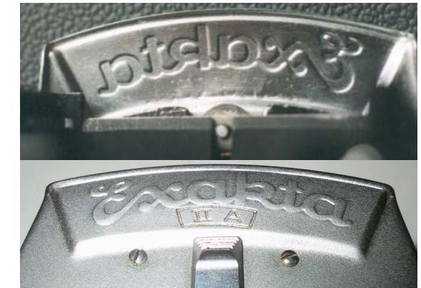
On the IIa the front plate was hammered under the embossed inscription "Varex IIa", then was professionally resilvered and then engraved. On the bottom the body number.
