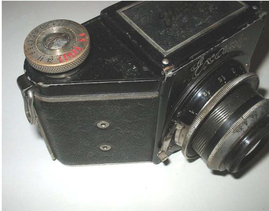
Lens lock on the right hand side while there is the (surely added) bipolar flash plug (like in the version 4). In the traditional version 2 there is the milled knob instead of lever, so I called this camera Version 2-3-4 (the 4 is for the bipolar plug). Cosmetically good, bad curtains (need to be replaced)
