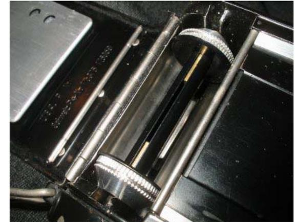
This camera is in bad functional condition, bad curtains, the lever doesn't reload the shutter, the ground glass is missing, mirror with some discoloration but cosmetically fine, good for display. I bought it because of its film window (professionally made) and take-up spools for 828 film, the same used by the Kodak Bantam cameras.
