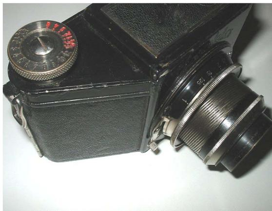
Lens lock on the right hand side while in the traditional version 2 there is the milled knob instead of lever, so I called this camera Version 2-3. Cosmetically fine, curtains pinholed even if the camera works well.
