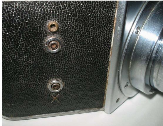
The two pins socket was replaced by two standardized synchro plugs. The owner engraves a X on the leather (for electronic). Probably the upper plug was for bulbs. The camera works fine and it is in fine condition.
