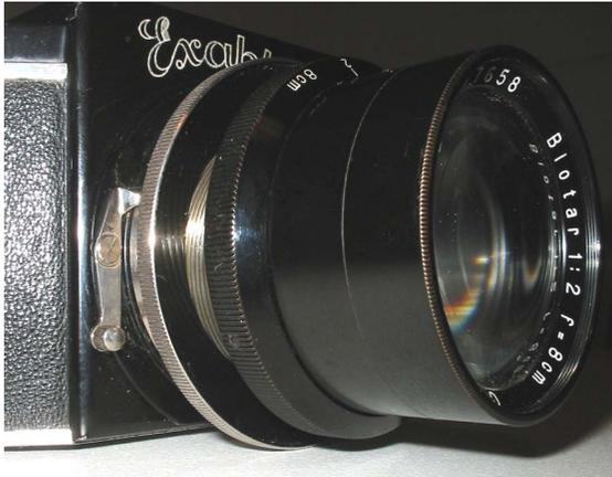
The locking lever for the infinity focusing position of the lens mount is on the right hand side, same body as the VP B version 2, with the Ihagee emblem on the viewfinder cover.
